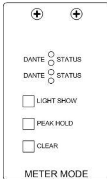
Figure 17: METER MODE/DANTE STATUS SECTION
